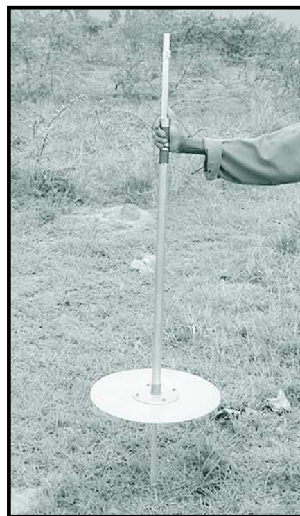
Figure 13.1: The Disc Pasture Meter developed by Bransby & Tainton (1977) used to estimate the standing crop of herbaceous plant material in a grass sward.
