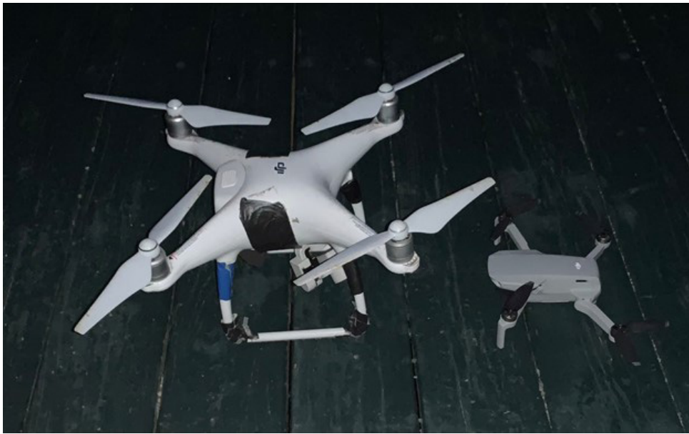
Figure 2. A wide variety of commercial drones are available. Three rotary quadcopters were used in this study, two of which are featured here. On the left, the DJI Phantom 4 was the largest and loudest drone used for this study. On the right, the DJI Mavic Mini was the smallest and quietest drone used for this study. Photo credit: Kayla Kuhlmann.
