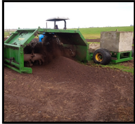
A compost-turner. Compost is turned on a daily basis for the first two weeks followed by turning every second day.
