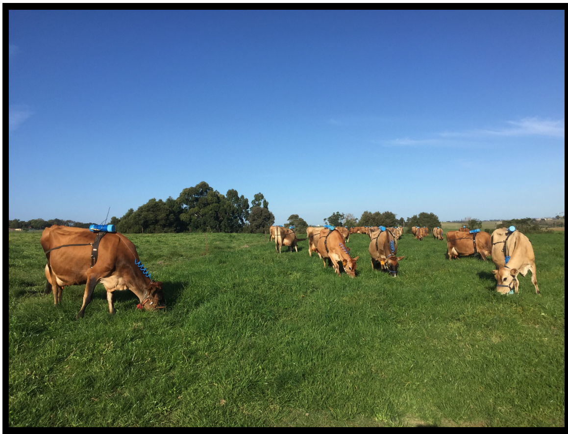
Methane research at Outeniqua research Farm: Jersey cows equipped with the SF6 technique on perennial ryegrass pasture.'
