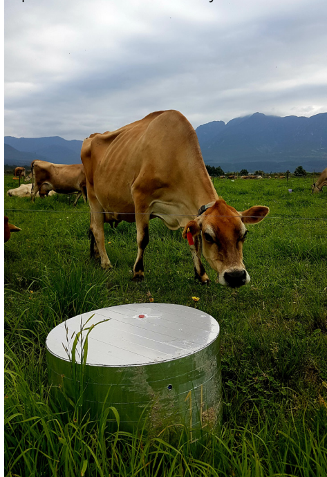
Figure 3: An example of the chambers used to collect gas samples in the current study.
