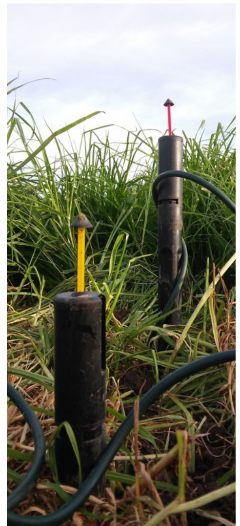
Picture 3: Fullstop™ Wetting Front Detectors show with red and yellow float indicate that a water sample is ready to be collected
