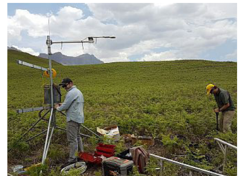
Figure 1: Byron Gray and Kent Lawrence install the Surface Renewal system in Catchment III, Cathedral Peak
