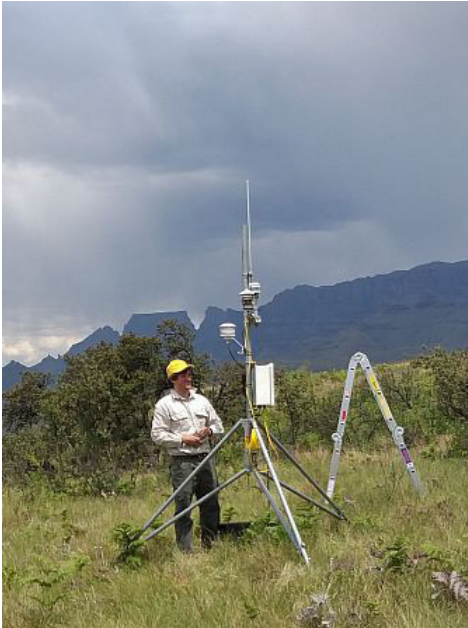
Figure 3: Byron Gray installs the Automatic Weather Station to support the Surface Renewal measurements in Catchment IX, Cathedral Peak
