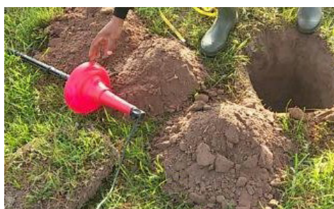
Picture 2: Inserting Fullstop™ Wetting Front Detector into the soil at 15 and 30 cm depths
