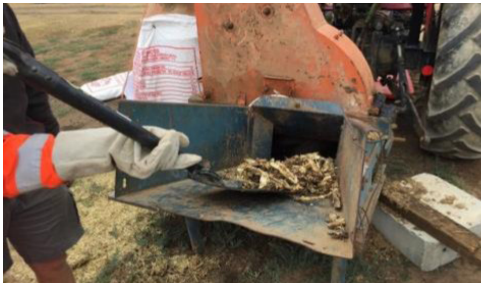
Photo 4: Grinding plant material in a hammer mill (photo: F Havenga)
